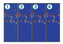
**Surface Noise**: Hides surface noise to help reduce clutter. Wider beam widths (lower frequencies) can show more targets, but can generate more surface noise.
