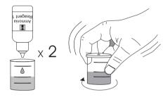
Add 8 drops of Nessler Reagent, replace the cap and mix by carefully swirling the beaker.
