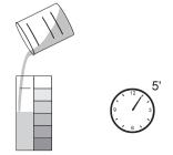
• Determine which color matches the solution in the cube, and record the results in ma/L (or ppm) NH.-N.
