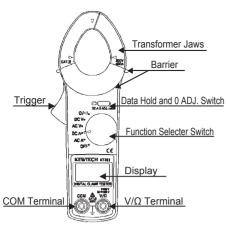
Barrier:It is a part providing protection against electrical shock and ensuring the minimum required air and creepage distances.
