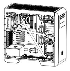
Connect the tubing and check all the fittings are sealed. The loop order: Pump Outlet > Water block
