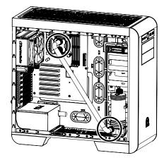
Connect the tubing and check all the fittings are sealed. The loop order: water black > radiator
