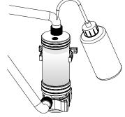
Place your PSU outside of the case and attach it to the pumps 4pin molex connector, turn on the power of PSU and make the rest of the system fills up.
