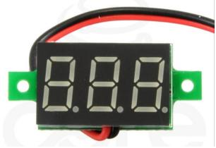
Applications include project power supply monitoring up to 30V while construction of DIY power supply project using along with Digital Display DC Ammeter (a separate device), monitor battery voltage of a car, motorcycle, truck or bus which have 12v /24v batteries. In addition, monitor UPS, Home Inverter Batteries of 12V/24V or Solar Panel voltage.
