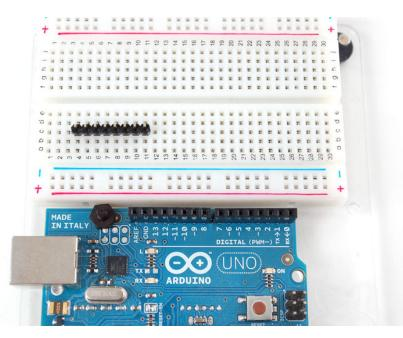
Slide either side of the LCD onto the header, the 'thicker' end is the top.
