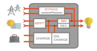
When PV output is reduced by clouds or at night, resulting in no surplus PV power available, loads powered by utility, batteries are charged, when utility outage, battereis are discharged.
