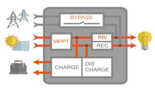
It combines a wide PV input range MPPT controller,can convert solar energy from PV to loads directly and the remaining solar energy converted to batteries synchronously.
