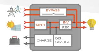
It can be running without batteries, energy shared from utility and solar to loads at the same time or alternatively.
